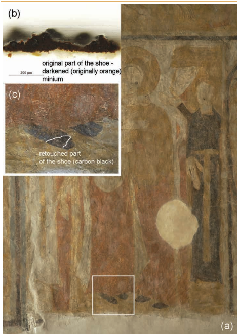
Fig. 5. Degradation and color change of minium ( Pb_3O_4 ). In the environment of dissociated carbonic acid minium disproportionates as follows: Pb_3O_4 (orange minium) + 2H_2CO_3 \rightarrow PbO_2 (brown-black plattnerite) + 2PbCO_3 (white cerussite) + 2H_2O ; this process of darkening is showed on the example of Pre-Romanesque murals in Slovakia (a), where some blackened parts of figures (b) were later retouched by carbon black (c) – not further respecting the original coloring.
