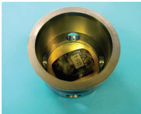
Fig. 2. Sample-holder for direct and non-destructive WDXRF analysis of a sillimanite adze from the Neolithic of Brittany (France). SCCYT, Cádiz University
