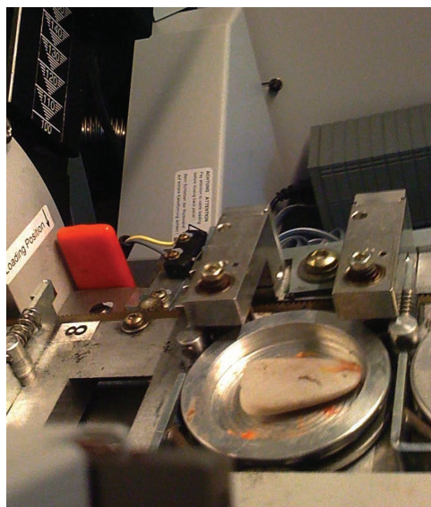
Fig. 1. Direct XRD analysis of archaeological objects. Sillimanite axe from a Neolithic site of Cadiz province, SW Spain. SCCYT, Cádiz University
