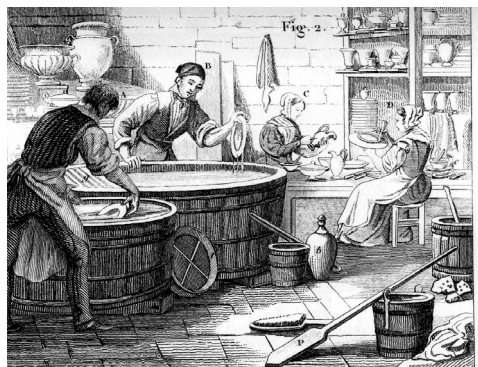
Fig. 14. Glazing and touching up. Two workers are dipping biscuit plates in the liquid containing the glaze powder. In the background, two female workers are touching up the raw glazed objects. The one in front is removing the glaze powder from the bottom of a plate with a brush or a piece of felt, so that it will not adhere to the support during firing, the other is removing with a blade the excess thickness of the glaze or their drops. (Brongniart, 1844, Plate XLVI).
