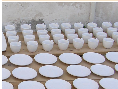
Fig. 15. Faience biscuits covered with raw white tin glaze, drying in the sun. Grottaglie, Italy. Photo M. Maggetti.
