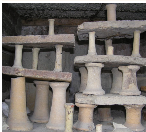
Fig. 19. Slabs, firing plates or shelves for placing wares in the kiln and columnar props or reels from the faience manufacture Le Bois d'Épense/Les Islettes (pers. coll.). Width of the slabs ca. 20 cm. Photo M. Maggetti.
