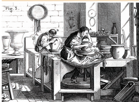
Fig. 9. Wheel throwing. The worker in front is shaping and his colleague behind is turning, i.e. finishing the object (Brongniart, 1844, plate XLV).
