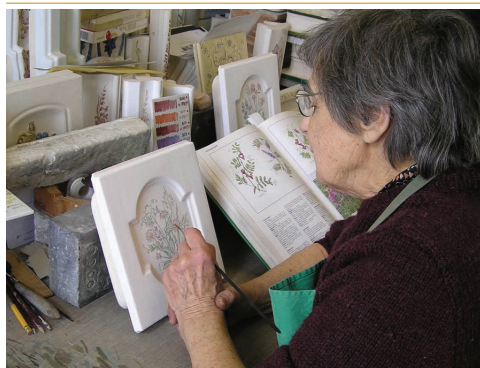
Fig. 17. In-glaze painting on tiles at the manufacture Schreiber Keramik AG, Matzingen, Switzerland. Photo M. Maggetti.
