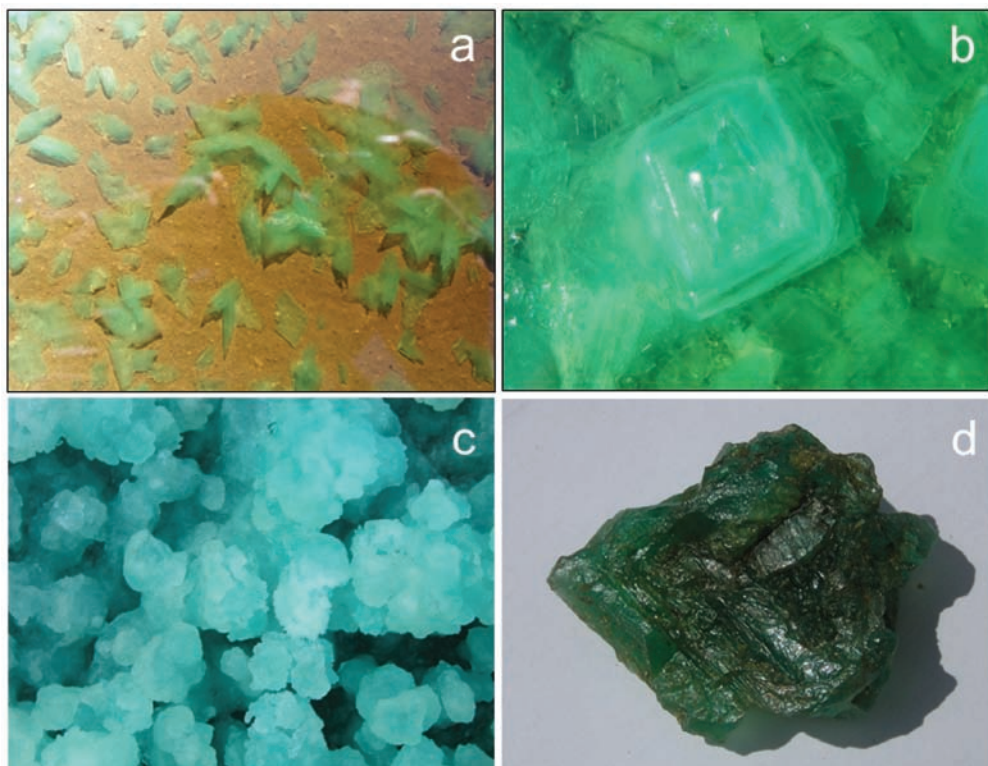
Fig. 12. (a-b) Emerald-green melanterite crystals formed in extremely acidic (pH 0.6) ferrous sulfate brine solutions in contact with fine-grained pyritic sludge in San Telmo mine (Huelva). Photo (a) courtesy of Dr. Francisco Velasco (UPV/EHU), (a-b) from Sánchez-España et al., (2008); (c) Cu-rich, blue-coloured melanterite crystals forming an efflorescence in the margins of an evaporating acidic stream in San Telmo mine; (d) Large crystal of rozenite formed in pore waters of a soil with pyritic sludge in Tharsis mine (Huelva). The fields of view are 10 cm (a), 2 cm (b), 5 cm (c), and 8 cm (d).
