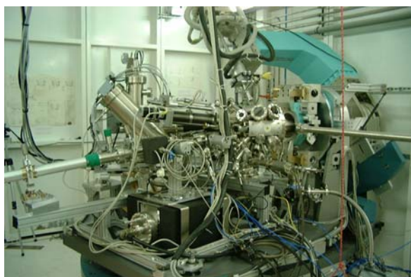
Figure 9. Photograph of the HAXPES and SXR experimental set-up installed at Branch B. It consists of a huge 2S+3D diffractometer, a UHV chamber with many surface science facilities and a high kinetic energy analyzer.
