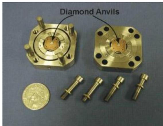
Figure 3: Parts of the Diamond anvil cell (from <http://www.crystal.vt.edu/crystal/dac.html>).
