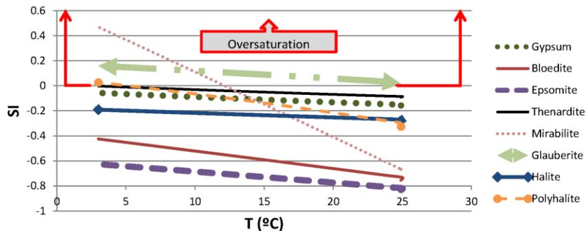
**Fig 1.** Saturation indices of the minerals while varying the temperature of the brine (Night and day). Only glauberite, mirabilite and Polyhalite are oversaturated.
