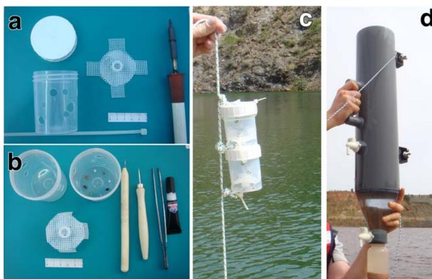
fig 1. Precipitation trap manufacturing with detailed holder and plastic net (a), mineral seeds mounted in the holder (b), aspect in field prior to submersion (c). Sample recovering from a sediment trap (d).
