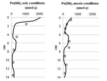
**fig 2.** Fe(III)-amorphous concentration in  $\mu$ mol/g under oxic (turnover, on the left) and anoxic (termocline, on the right) conditions versus depth (cm). The points correspond to analytical data and the line to the model results.
