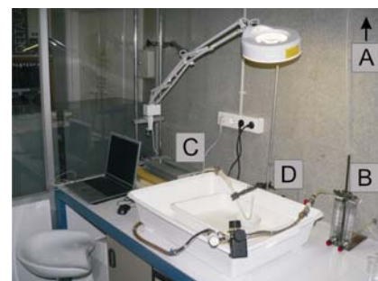
fig 2. HS 11 system at the University of Barcelona; A: water tank for gravity flow out of sight; B: flowmeters; C: HS11 device with connected laptop; D: Glass-Separation-Tube (GST).
