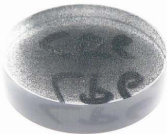
fig 4. Closely-packed monolayer polished section of final concentrate; diameter = 2.5 cm.
