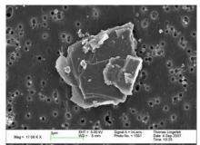
fig.1 Typical mineral road dust particle
