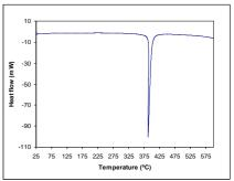
fig 1. DSC heating process of the azurite pigment.
