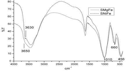
fig. 2. FT-IR Spectra of samples SMgFe and NiFe.
