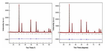
**Fig. 1.** Observed (dots) calculated (solid line) and difference X-ray diffraction profiles for  $[Eu_{2x}Mg_x][Sn_{2x}Mg_x]O_{7:3x/2}$  (left) and  $[Eu_{2x}Zn_x][Sn_{2x}Zn_x]O_{7:3x/2}$  (right). Vertical marks correspond to the allowed reflections for the space group Fd-3m.
