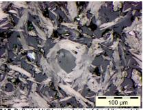
fig 5. Reflected light micrograph of graphite crystals
