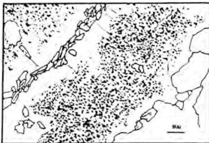
Fig.1 - Distribution of fluid inclusions in the alkali feldspars : very abundant in the cores, but never observed in the rims of the crystals.
