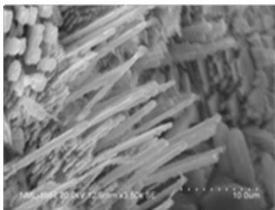
fig 2b. SEM image of As(III) doped lepidocrocite
