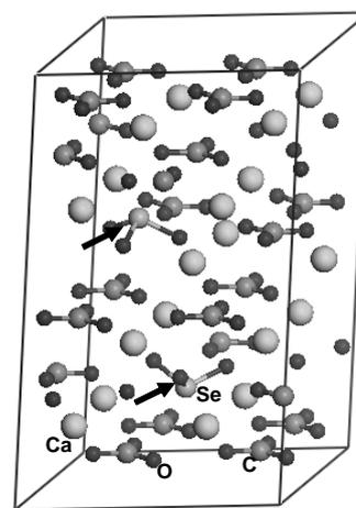
**fig 1.** Simulated incorporation of selenite molecules  $\text{SeO}_3^{2-}$  in the calcite unit cell. The arrows show the two Se atoms which were placed at a carbon site in the initial stages of the simulation and evolved to adopt a pyramidal configuration.
