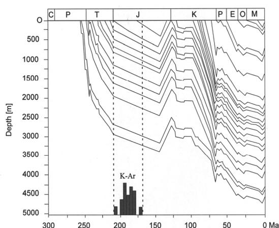
FIGURE 8. K-Ar data of authigenic illite from Rotliegende sandstones in northern Germany relative to the reconstructed burial history of the sediments; the results are far from maximum burial seen from simulated burial curves (after Zwingmann et al., 1999).
