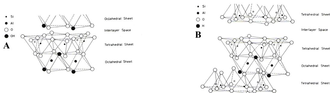
FIGURE 1. *A: Crystal structure of a 1:1 type clay mineral. B: Crystal structure of a 2:1 type clay mineral.*
