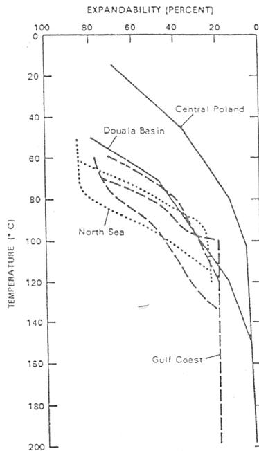
FIGURE 12. *Expandability factors of illite-smectite mixed-layers from sediments of varied basins relative to burial (= temperature) increase.*
