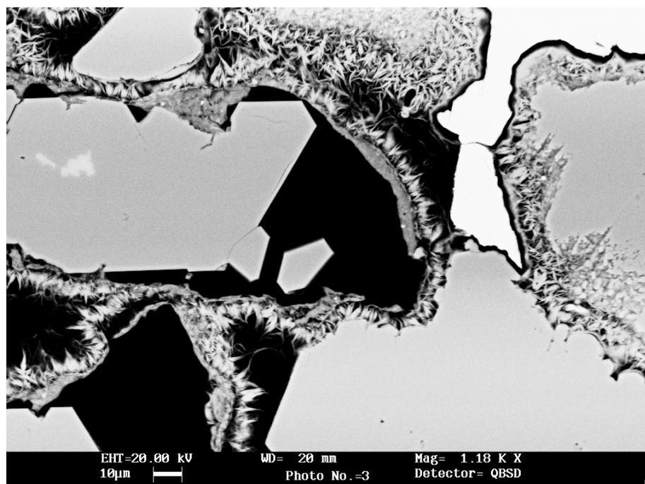
FIGURE 2. Scanning photograph of a sandstone consisting in quartz grains (grey), siderite (white) and large pore spaces (in black) filled with authigenic illite-type clay material (Courtesy of ARAMCO).
