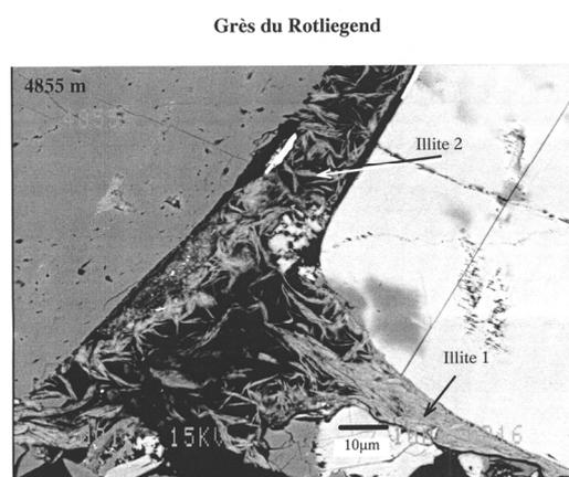
FIGURE 9. Authigenic illite in the pore system of a Rotliegende sandstone from northern Germany; illite 1 is palisadic and illite 2 is fibrous (after Liewig and Clauer, 2000).
