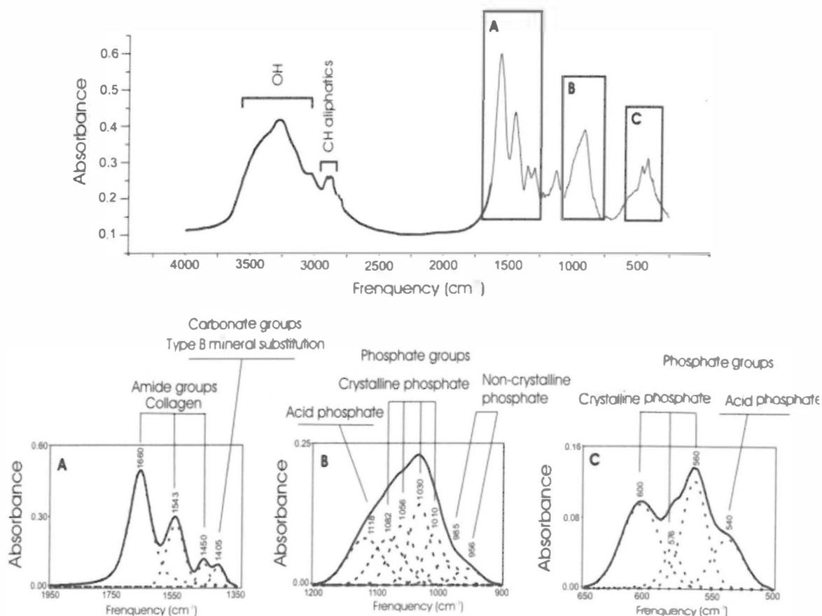
Figure 1: FTIR spectra of bone samples (400-4000  $\text{cm}^{-1}$ ) and overlapping peaks constituting the main band regions determined. Peaks position information was collected from the references: Paschalis et al. 1996, Boskey 1999, Bohic et al. 2000, Miller et al. 2001.
