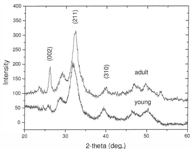
Figure 2: X-ray diffraction pattern from Clapper Rail leg bone characteristic of apatite with broad peaks typical of the nanocrystalline nature of bone mineral.
