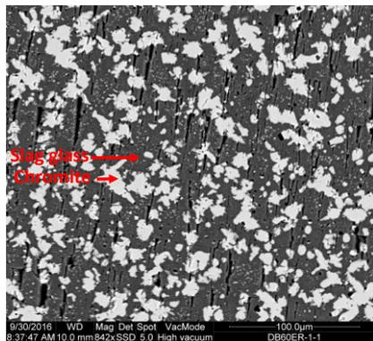
fig 3. Backscattered electron (BSE) image of electrofused magnesio-chromite. In white=chromite; in dark=slag glass.
