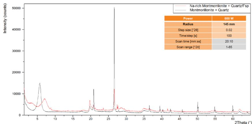
fig 8. Clay mineral scans obtained with compact diffractometer in 20 minutes measuring time.
