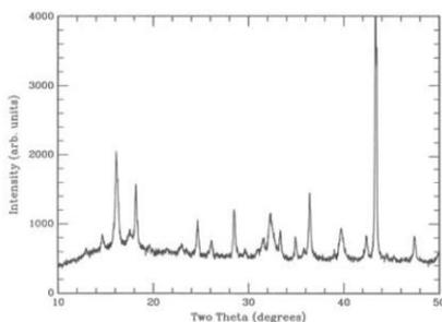
fig 4. Original graphic of the X-Ray diffraction pattern of a rust sample published in *Powder Diffraction* 1, 299 (1986).
