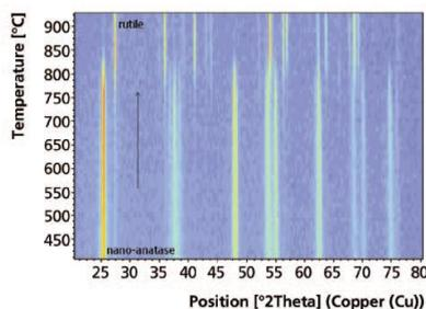
fig 1. Isolines plot showing the thermal evolution of XRD patterns with an increasing intensity from blue (background) to yellow and orange (Bragg Peaks)
