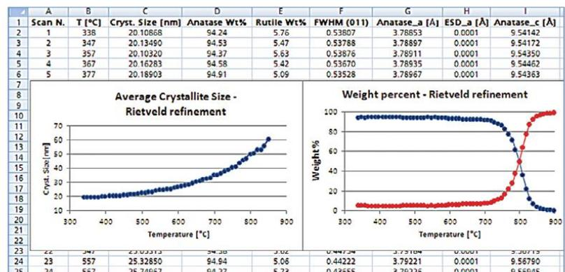
fig 3. Output of automatic analysis with refined parameters and corresponding plots
