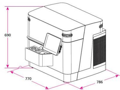
fig 7. Compact diffractometer dimensions
