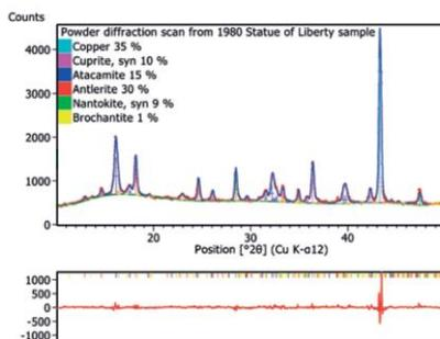
fig 5. Rietveld refinement performed on the converted scan.
