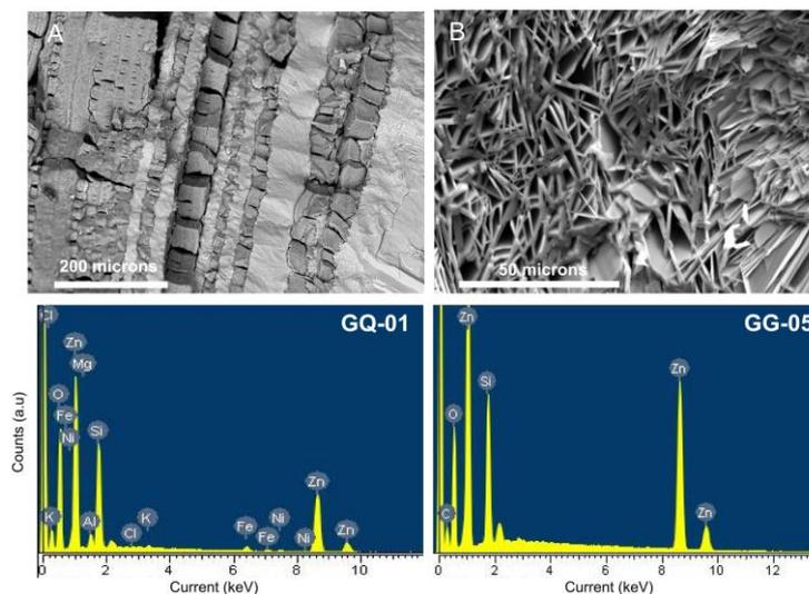
fig 3. SEM images of samples GQ-01 (A) and GG-05 (B), and their corresponding EDX spectra.
