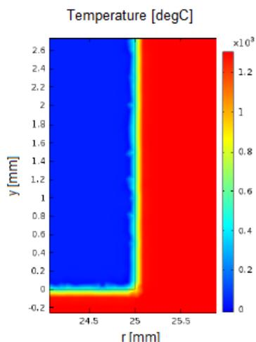
fig 3. Temperature distribution at  $t = 0$  seen across an axial cross-section through the sampler.
