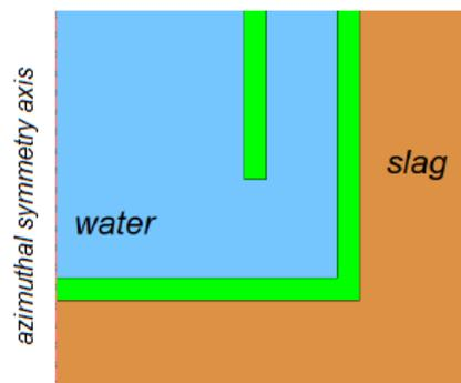
fig 1. Sampler axial cross section.
