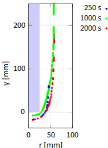
fig 4. Isothermal lines recorded for 1100 °C around the sampler at various times after the immersion of the sampler into the slag layer.
