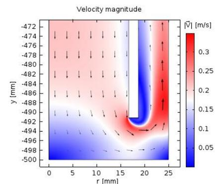
fig 2. Water velocity distribution across sampler axial cross section.
