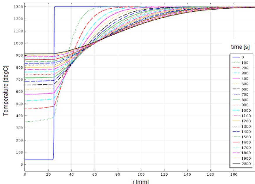
fig 5. Time temperature evolution across sampler and slag domains. Time range goes from 0 to 2000 s. Initial temperature within sampler is 40 °C and temperature of slag around sampler is 1300 °C.
