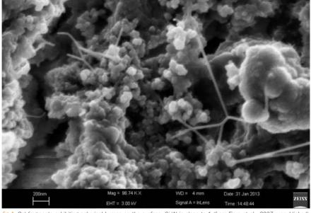
fig 4. Gel fragments exhibiting spherical humps on the surface. Si/Al is close to 1 (from Fiore et al., 2007; unpublished). SEM image.
