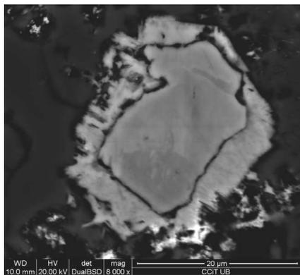
**fig 3.** Nb-bearing rutile partly replaced along grain rims by goethite. Slighter areas in the rutile core correspond to Nb-rich domains. SEM-BSE image.
