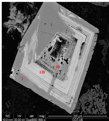
**fig 2.** Complex internal texture of a pyrochlore crystal from Bailundo. A Pb-rich secondary pyrochlore (13b) replaced completely the crystal along the primary zoning, and a late generation with Ca-Na-F rich pyrochlore (1) replaces all the above generations along the grain rims and cracks. SEM-BSE image.
