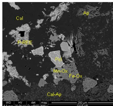
**fig. 1.** SEM-BSE image of a sample of an altered carbonatite from the center of the Bailundo carbonatite complex, showing primary and secondary phases. Mineral abbreviations: Pcl: pseudomorphs of euhedral primary pyrochlore, Ap: primary apatite, Cal: calcite, MnOx: secondary Mn-oxide, FeOx: secondary Fe-hydroxides pseudomorphic after magnetite crystals. Cal-Ap: fine intergrowths of secondary carbonates with secondary apatite. PREE: Late REE phosphates.
