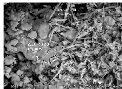
fig 2. Calcium (aluminite) silicate hydrates (CASH) needles and fibers (SEM).
