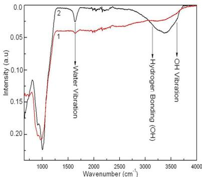
fig 4. ATR-FTIR Infrared Spectra of Pillow Lava. (1) Internal Surface of the Sample (2) External Surface of the Sample.
