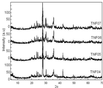
fig 3. XRD Diffractograms of the Pillow Lavas Samples.
