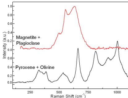
fig 2. Raman Spectrum of Pillow Lava. Shown two spectra of the crystal matrix. The Original fluorescence was corrected.
