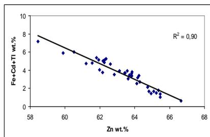
Fig. 2. Negative correlation between Zn and Fe+Cd+Tl in the sphalerite from the El Losar del Barco mine.
