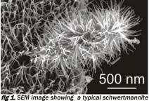
**fig 1**. SEM image showing a typical schwertmannite hedge hog that can be easily misinterpreted as a bacteria cell that was overgrown by schwertmannite whiskers.
