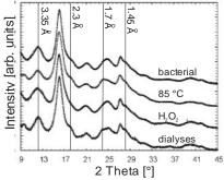
fig 2. Diffractograms of schwertmannites that were synthesized in different conditions. The obtained diffractograms differ in intensity as well as peak broadening of several marked reflections. The used wavelength was 0.709 Å (Mo K $\alpha$ ).
