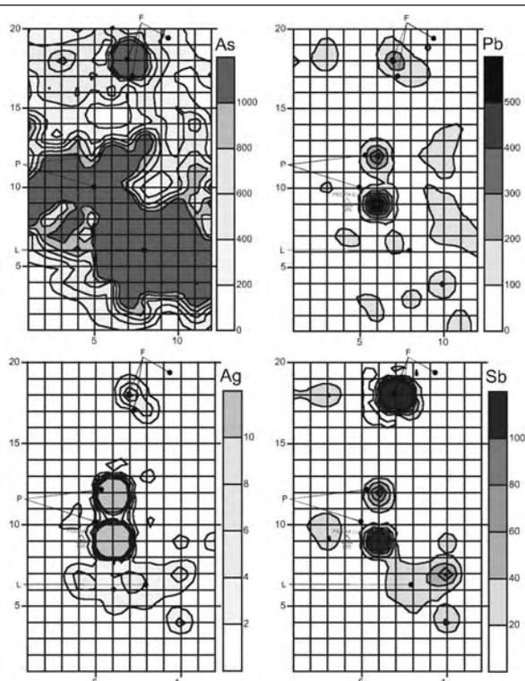
Fig. 1. Distribution of As, Pb, Sb and Ag in soils (mg/kg) of Freixeda region. Grids has 200 meters per side. F – Freixeda tailings; P – Pedra Luz tailings; L – Lombo Veiga tailings.
