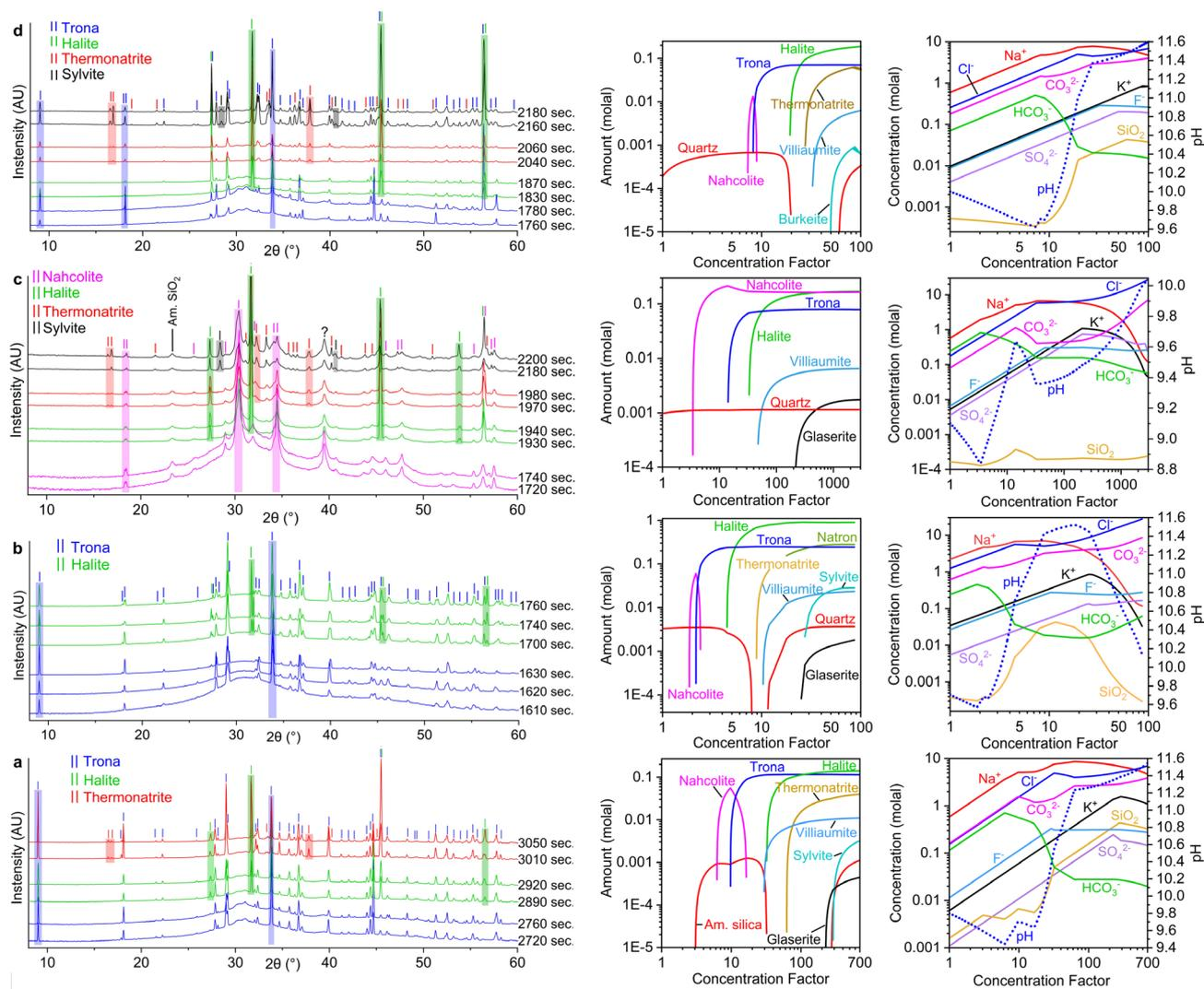
**Fig 1.** Powder X-ray diffraction data from *in-situ* (levitated drop) evaporation /precipitation experiments of (a) Lake Magadi brine, (b) Lake Nasikie Engida brine, (c) Nasikie Engida hot spring and (d) Lake Natron brine (left column). Simulation of the same process by hydrochemical modeling; precipitated mineral phase amounts and solution species concentrations are represented as a function of the concentration factor (initial solution weight divided by the current solution weight).
