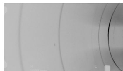
fig. 1 XRD pattern collected on the Imaging Plate corresponding to yellow sample (yellow type I) from the Bargello work.
