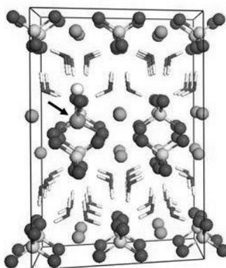
**fig 2.** Incorporation of an arsenate molecule  $\text{HAsO}_4^{2-}$  in the gypsum unit cell. The arrow shows As atom.
