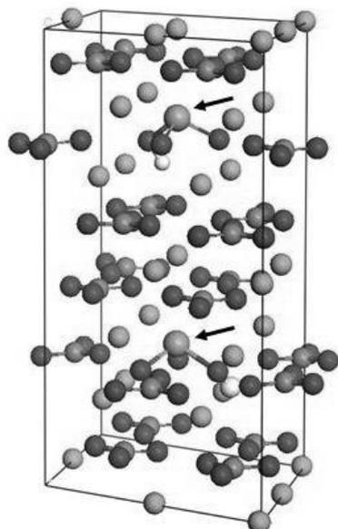
**fig 1.** Incorporation of an arsenite molecule  $\text{HAsO}_3^{2-}$  in the calcite unit cell. The arrows show As atoms.
