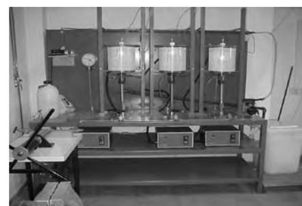
fig 1. General view of the SIMGEO experimental laboratory where can be observed the three cold seal vessels, their furnaces and the accessory equipment.
