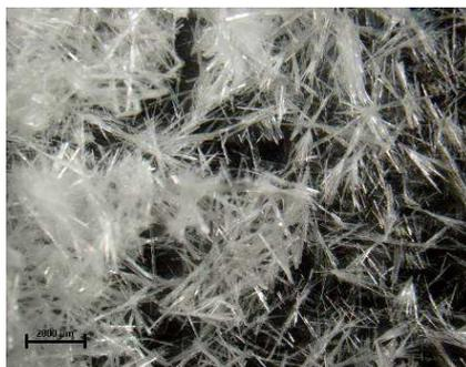
Fig. 1 Gypsum crystals grown at 40 °C.
