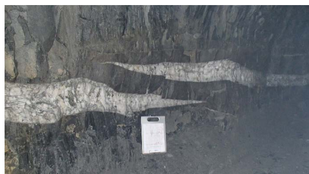
Fig 2. Example of a mineralized vein ending as an “eel tail”. (Source: photography from the authors).
