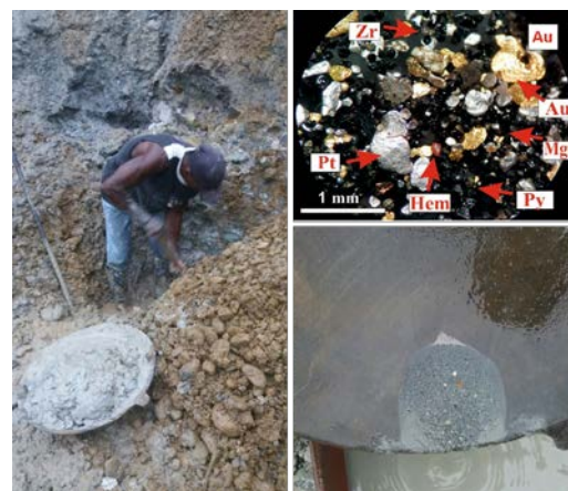
Fig 4. Example of artisanal small-scale mining from placer sediments in South-America. Pt-bearing minerals ("Pt-Fe nuggets", labelled as "pt" in figure) and Au are concentrated via panning ("gold washing") together with other typical heavy minerals such as zircon (zr), magnetite (mgt), hematite (hem) and pyrite (py).
