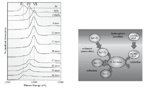
FIGURE 9. Left: Se K-edge spectra of culture after 0, 12, 21, 28, 37, 43, 53 and 66 hours from seeding S. barnesii, along with Se,  $SeO_2$  and  $CaSeO_4$  for reference. Right: Pattern diagrams of dynamics of selenium in aquatic sediments.
