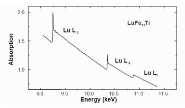
FIGURE 1. X-ray absorption spectra of LuFe<sub>11</sub>Ti at the Lu L-edges, involving different final state symmetry:  $L_3 (2p_{3/2} \rightarrow \varepsilon \{ d_{3/2}, d_{5/2} \}), L_2 (2p_{1/2} \rightarrow \varepsilon d_{3/2}), L_1(2s_{1/2} \rightarrow \varepsilon \{ p_{1/2}, p_{3/2} \}).$
