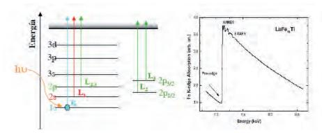
FIGURE 2. Schee of the excitation of an electron by the absorption of a x-ray photon.
