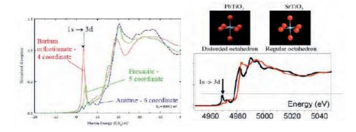
FIGURE 6. Ti K-edge XANES spectra of reference compounds in which Ti ion shows the same oxidation state but different coordination.
