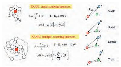
FIGURE 4. Single and multiple-scattering processes in x-ray absorption.
