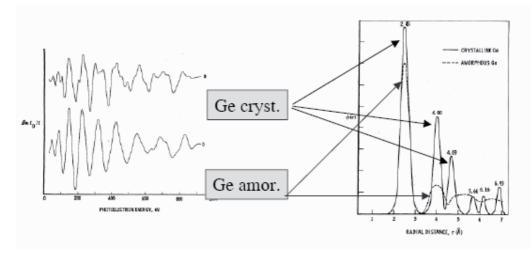
FIGURE 7. Ge K-edge EXAFS spectra and their Fourier transforms in the case of crystalline and amorphous Germanium.
