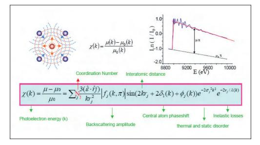
FIGURE 3. Schematic illustration of the interference phenomena giving rise to the modulations (EXAFS) in the x-ray absorption cross-section.
