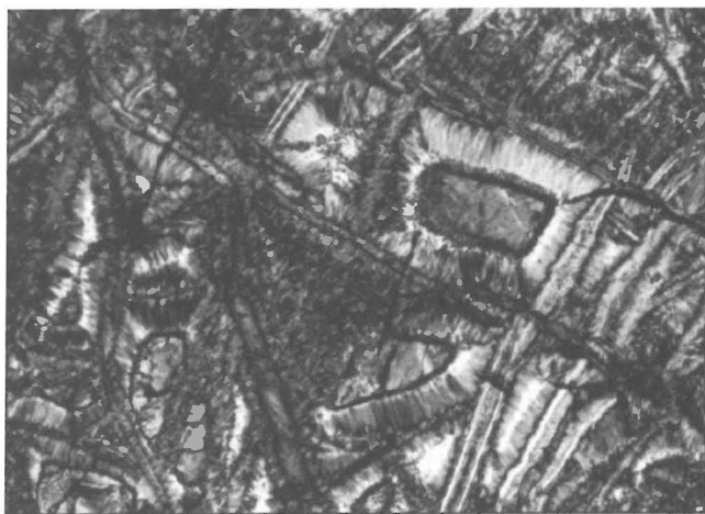
Figura 1: Mesh texture of lizardite around olivine relicts. Polarizing microscope image between crossed nicols. Bigger olivine grain = 0.3 mm.
