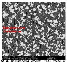
**rig 3.** Backscattered electron (BSE) image of electrofused magnesio-chromite. In white=chromite; in dark=slag glass.
