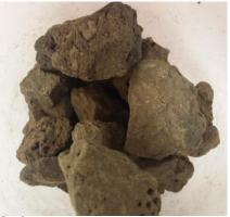
fig 2. Electrofused Magnesio-Chromite as raw material for industrial refractory making.
