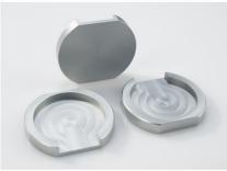
fig 6. Example of side loading holders
