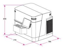
fig 7. Compact diffractometer dimensions
