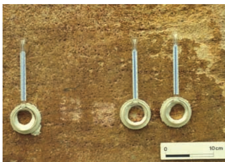
fig 20. Water uptake measurements with Karsten tubes.
