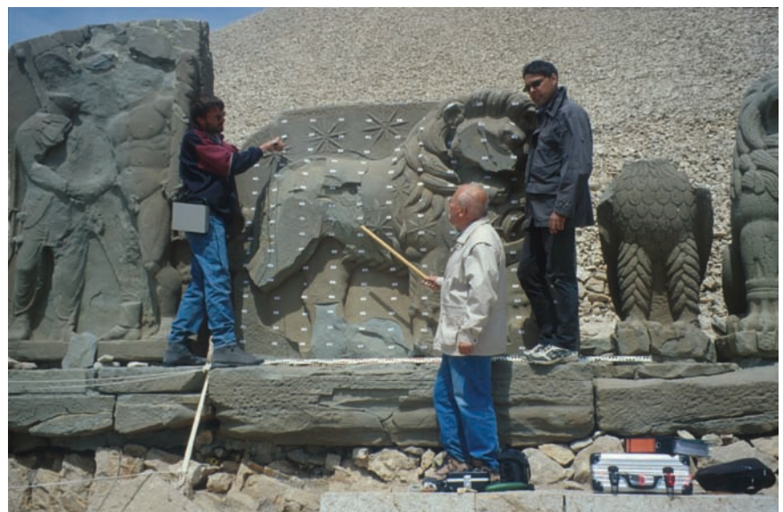
fig 18. Ultrasonic measurements, lion horoscope / Nemrut Dag (Turkey).
