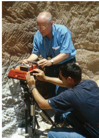
fig 22. Drilling resistance measurements.
