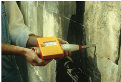
fig 21. Rebound hardness measurements, Schmidt hammer.
