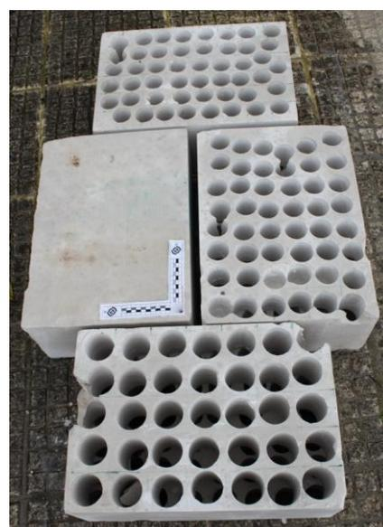
fig 1. Rock blocks of the Corvio Sandstone after core plug extraction.
