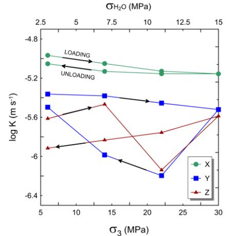
fig 3. Log hydraulic conductivity vs. confining ( $\sigma_3$ ) and pore ( $\sigma_{H_2O}$ ) pressures of three Corvicio Sandstone plugs sampled in orthogonal directions: X and Y parallel to bedding and Z at right angle.
