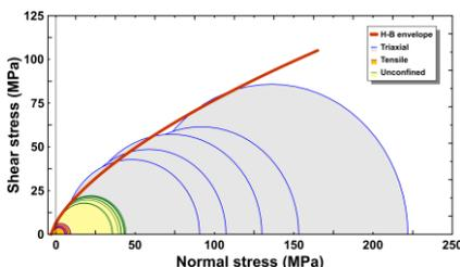
fig 2. Mohr circles corresponding to the different mechanical tests performed (Brazilian, UCS and triaxial) with the Corvicio Sandstone. The computed Hoek-Brown strength envelope computed from these tests is also shown.
