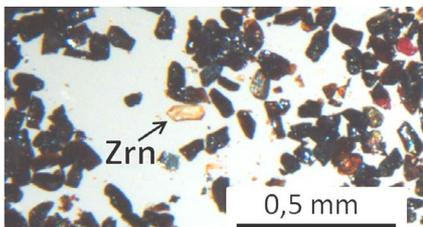
fig 3. Final concentrate (size fraction  $< 53\mu\text{m}$ ) with zircon (Zrn) observed by binocular microscope.
