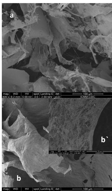
**fig 2**: FE-SEM images of (a) sacran polysaccharide and (b) the bionanocomposite sacran-sepiolite with 17 wt% of sepiolite.
