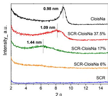
**fig 1** : XRD patterns of pristine sacran and Clois-Na, and the bionanocomposites resulting from their assembly.
