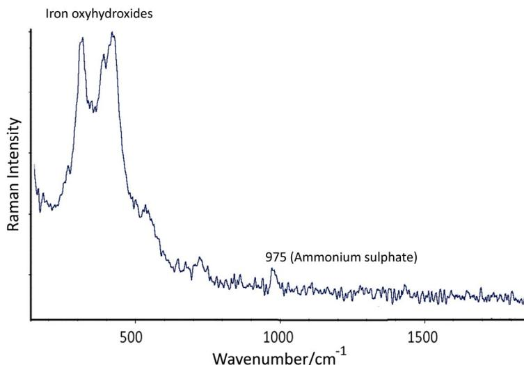
fig 1. Raman spectra of ammonia sulphate in a steel surface.
