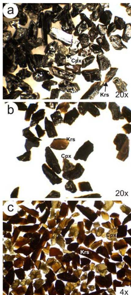
**Fig. 1.** Microphotographs of the 3200-3300 kg/m<sup>3</sup> density and 410-500 mA current intensity magnetic susceptibility fraction on a transparent tray under the petrographic microscope, plane polarized light. a) 400-500 µm fraction. b) 400-500 µm fraction, with ethanol. c) 250-300 µm fraction, with acetone and tracing paper; note the easily recognizable brown and light-green colours in this photograph, in spite of its lower magnification.
