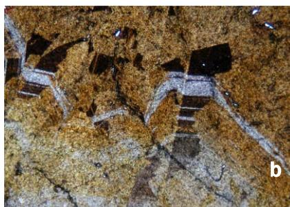
Fig. 1. Photomicrographs in polarized transmitted light (PP 2.5X) of cracked banded-sphalerite (a) and twinned sphalerite with relicts of zonation (b).
