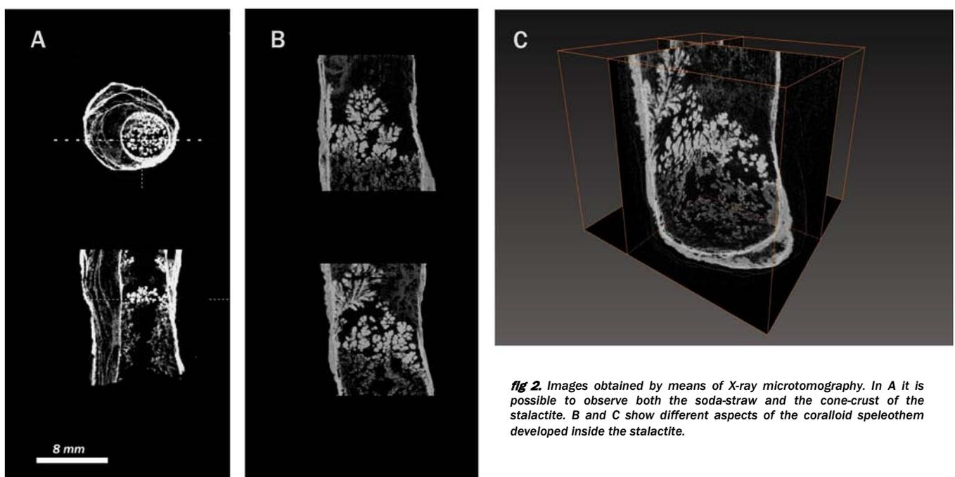
**fig 2.** Images obtained by means of X-ray microtomography. In A it is possible to observe both the soda-straw and the cone-crust of the stalactite. B and C show different aspects of the coralloid speleothem developed inside the stalactite.
